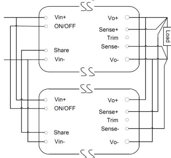
**Figure 6.** Circuit Configuration for Active Current Share
