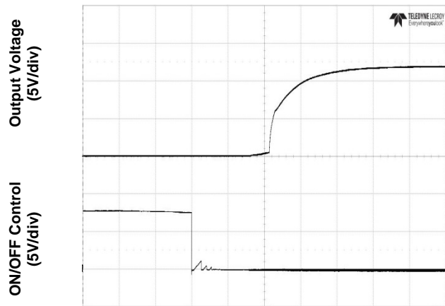
Figure 4. Start-Up from Enable Control (typical Vin, full load)
