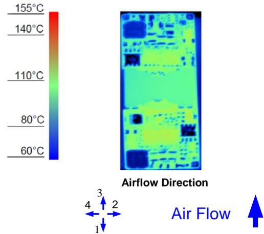
**Figure 10.** Thermal Image for Airflow Direction 3 (5A output, 55°C ambient, 200 LFM, typical Vin, open frame, unit soldered onto a fixture board)
